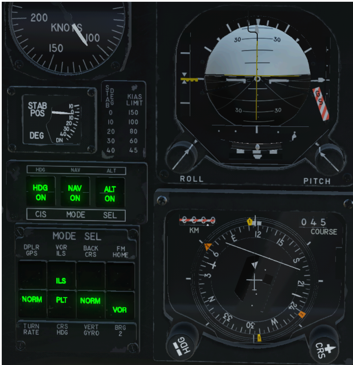
ILS Heading submode - note HDG ON light and Roll Command Bar following set Heading Bug bearing. ALT ON light indicates Collective Command Bar is maintaining Altitude Hold submode
