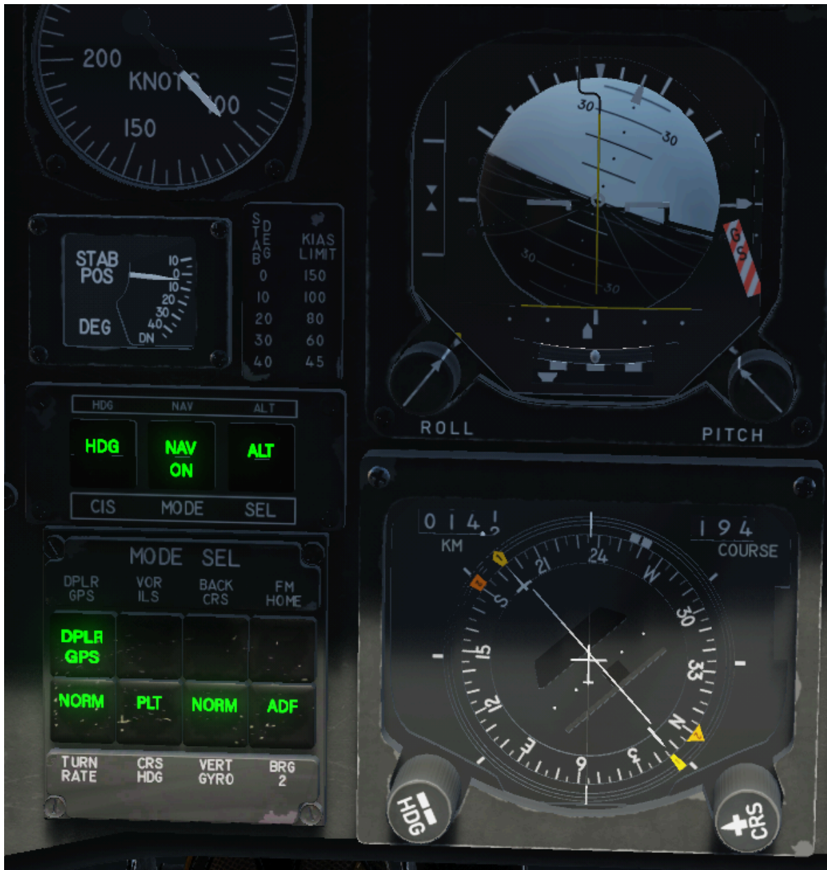
Intercepting the FLY TO course. Note the Course Pointer has been aligned to the Number 1 Pointer manually to aid visual indication of the course and deviation
