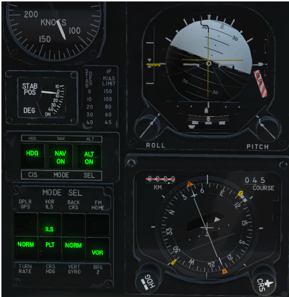
Intercepting the ILS radial - note HDG ON light extinguished
