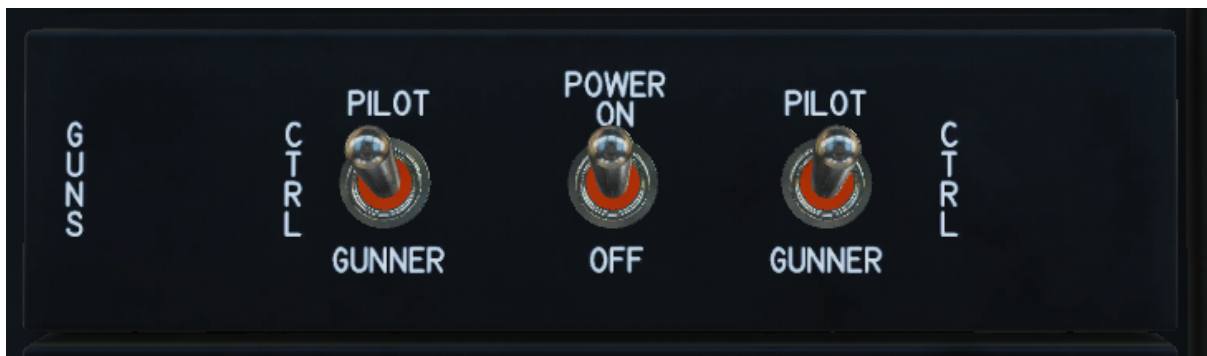
Door Guns Control Panel with power applied and guns in Pilot control mode
