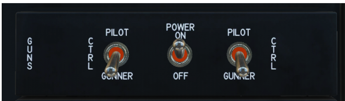
Door Guns Control Panel with power applied and guns in Gunner control mode
