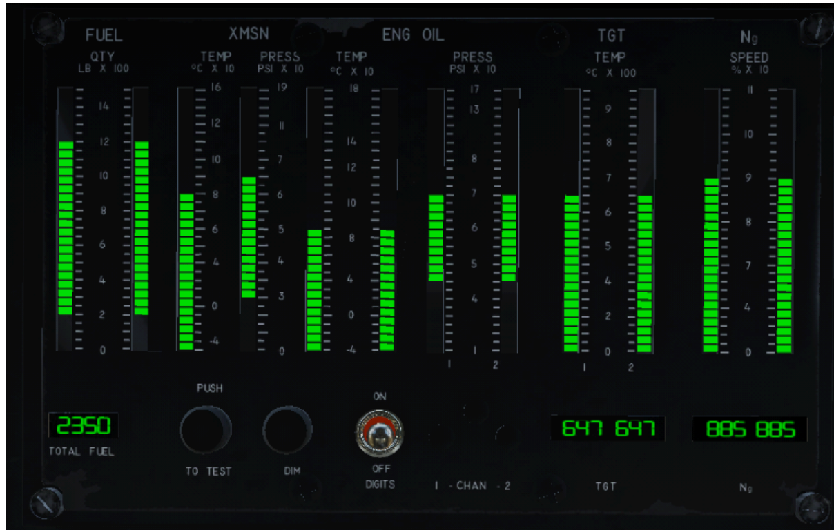
Internal fuel quantities displayed on the left side on the Central Display Unit
