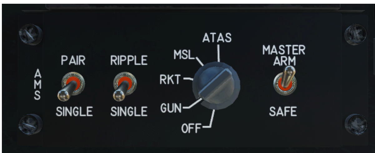
Armament Management System with GUN selected and Master Arm ARMED
