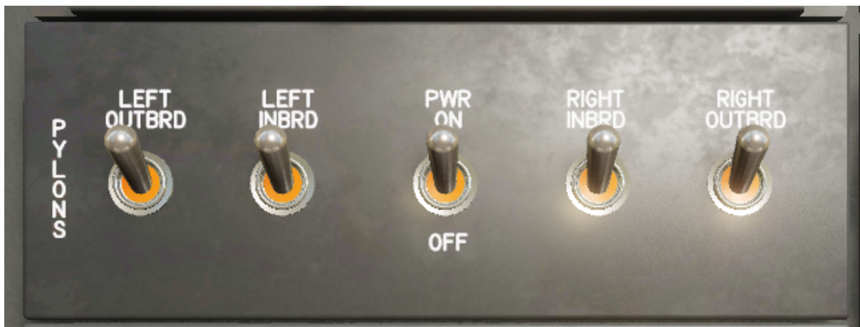
Pylon Power Control Panel with power ON and all pylons selected
