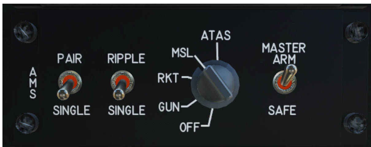
Armament Management System with MSL selected and Master Arm ARMED.
