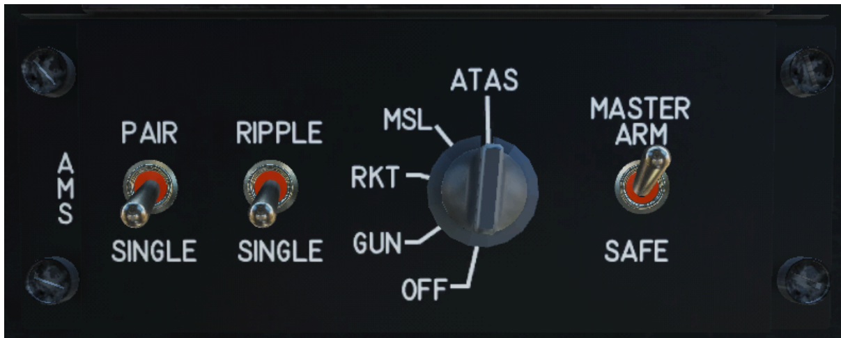
Armament Management System with ATAS selected and Master Arm ARMED.
