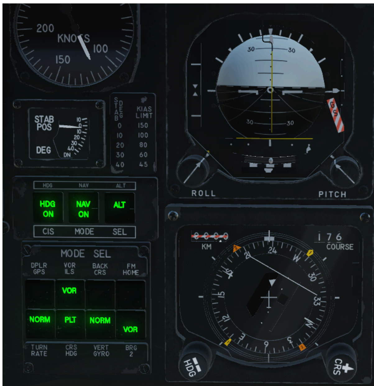
VOR Heading Submode - note HDG ON and Roll Command Bar directing to Heading Bug
